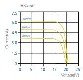
Note: all electrical parameters are rated at standard test conditioins (irradiance of 1000W/m2 , AM 1.5G, cell temp.  $77^{\circ}F/2$
