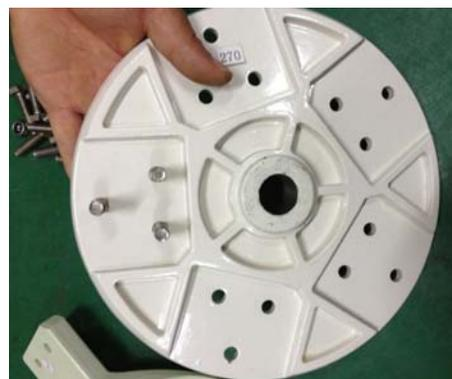
⑤ Place blade, flat washer and nylock nut, and tighten the nut to 18N.m
