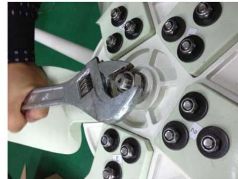
③ Fully tighten the nut to 154N.m
