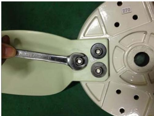
④ Pass the hex bolts through from the back side of the hub.
